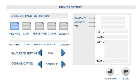
We can choose the suitable baud rate and communication style for different print or connect with the computer.
