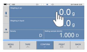
When the weighing digit value stable, press again then will be show green square. Means confirm the weight in the air.
