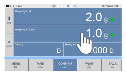
Step 4: Press the density, the result will be come out, the density unit is g/cm<sup>3</sup>
