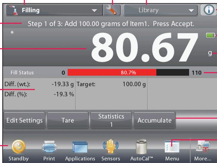
Battery life indicator when powered by optional battery pack (for High Capacity models only)
