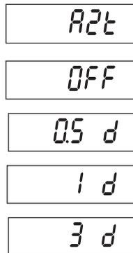
**NOTE:** When the LFT menu item is set to ON, the selections are limited to 0.5d and 3d. The setting is locked when the hardware lock switch is set to the ON position.
